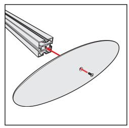
Base Plate & Extrusion Connection
